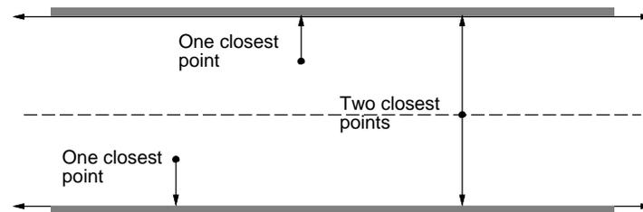
Figure 6.8: The maximum clearance roadmap keeps as far away from the  $\mathcal{C}_{obs}$  as possible. This involves traveling along points that are equidistant from two or more points on the boundary of  $\mathcal{C}_{obs}$ .
