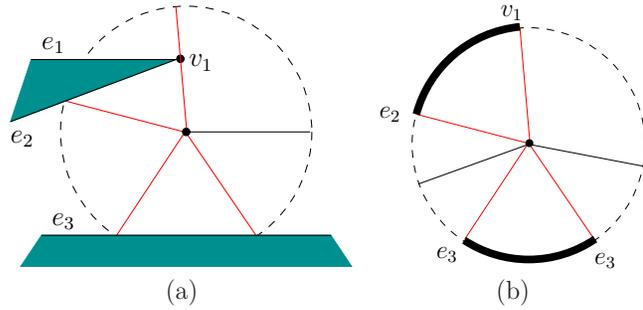
Figure 6.22: Fix  $(x, y)$  and swing the segment around for all values of  $\theta \in [0, 2\pi]/\sim$ . (a) Note the vertex and edge features that are hit by the segment. (b) Record orientation intervals over which the robot is not in collision.
