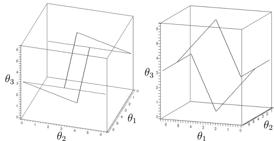
Figure 4.26: If two constraints,  $f_1 = 1$  and  $f_2 = 0$ , are imposed, then the varieties are intersected to obtain a 1D set of solutions. The example is equivalent to a well-studied four-bar mechanism.
