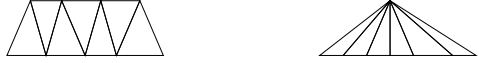
Figure 3.6: Triangle strips and triangle fans can reduce the number of redundant points.
