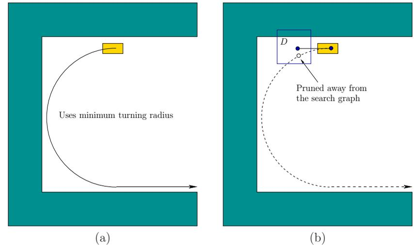
Figure 14.18: (a) The Dubins car is able to turn around if it turns left as sharply as possible. (b) Unfortunately, the required vertex is pruned because one cell along the required trajectory already contains a vertex. This illustrates how missing a possible action can cause serious problems many stages later.
